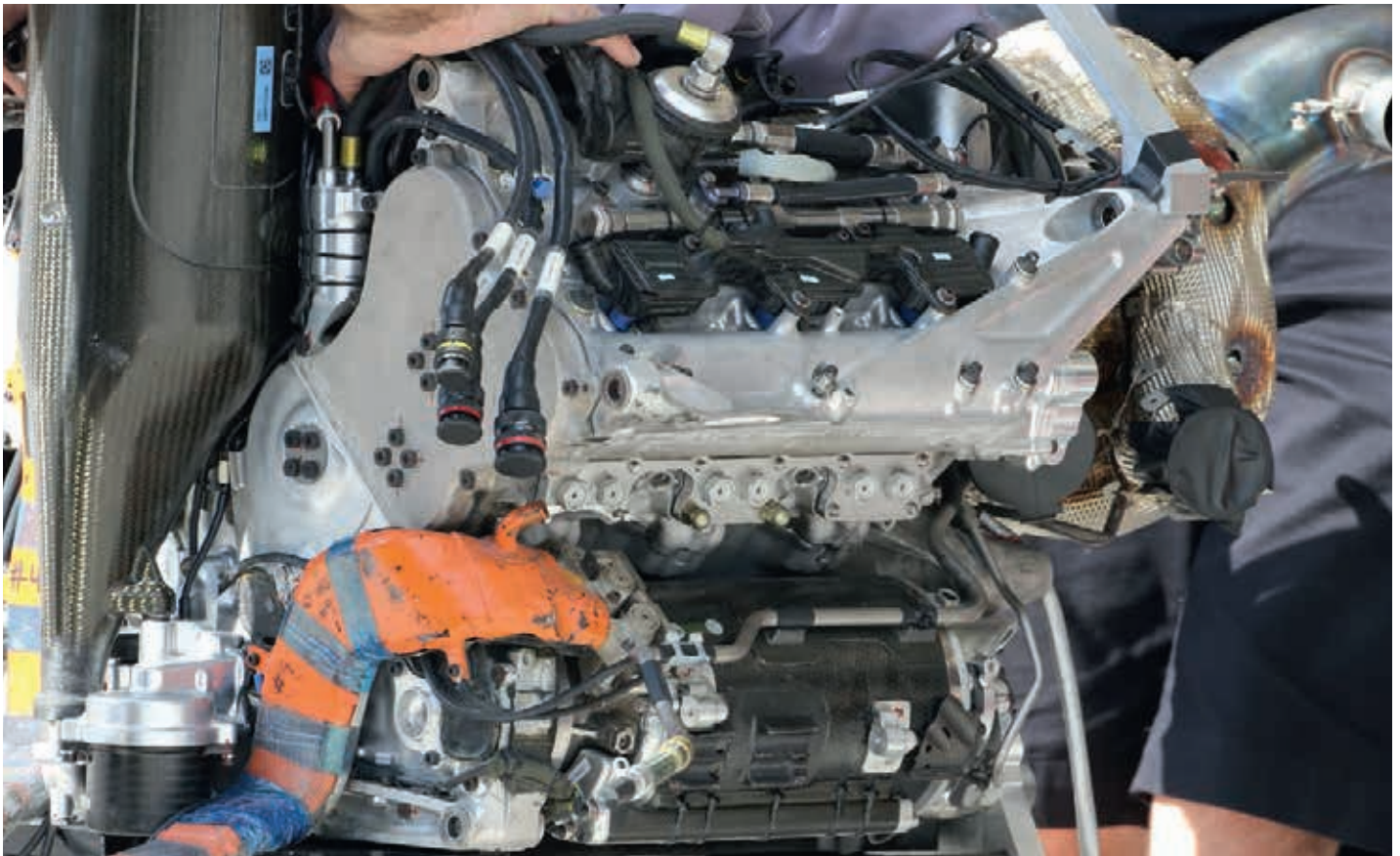
A picture of the 2014 V6 engine for the purpose of comparison – it looks as though it has a different MGU-K and turbine entry. This engine powered Red Bull to three wins last year
