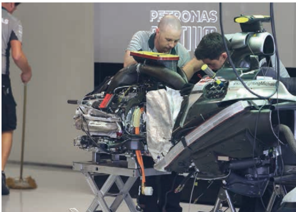
The 2014 power unit in the Mercedes W05 – the much smaller plenum is clear in this pic, as is the smaller exhaust header
