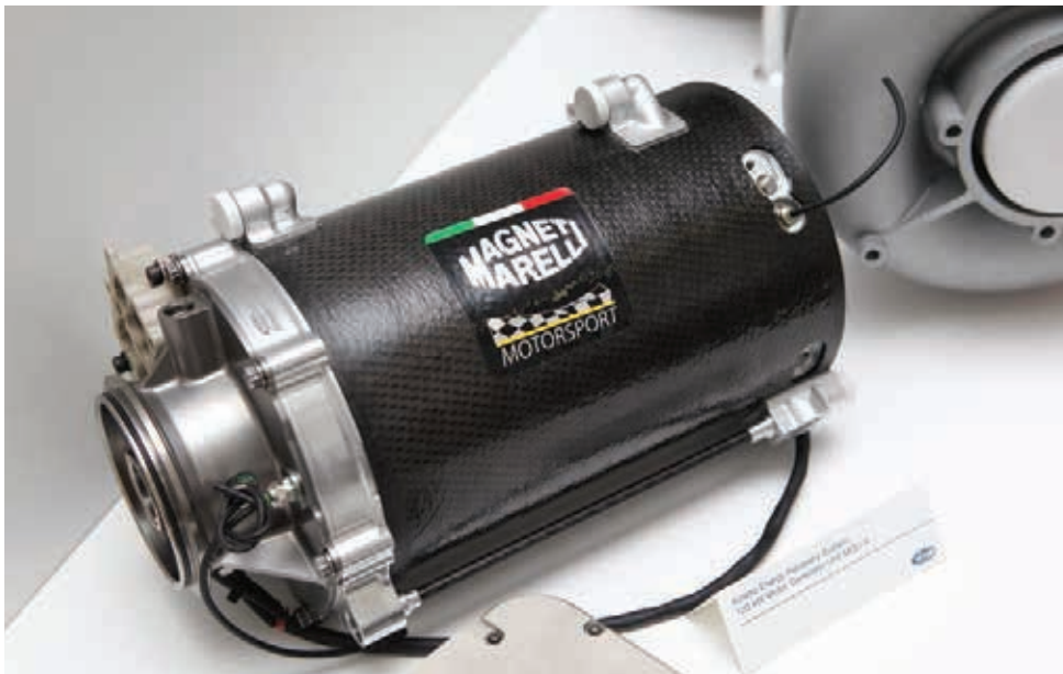
Magneti Marelli MGU-K can pack 120kW and 450v and weighs 10kg – which seems a fair trade off when all's said and done
