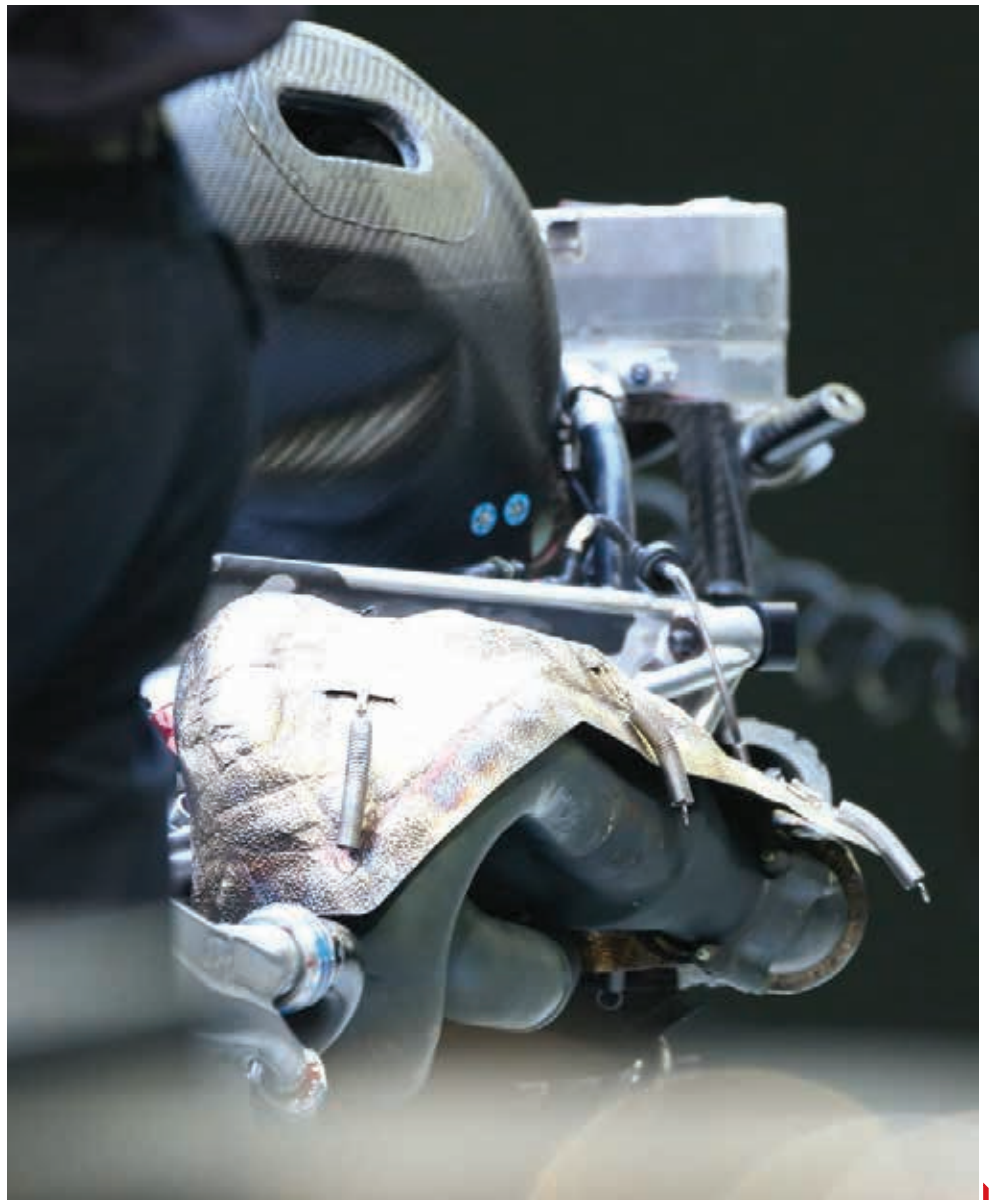
PU106B exhaust system features longer primaries, increasing the size and mass of the design but also the power output
